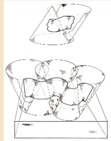
MultiConic Patent drawing: Flat surface material can be easily curved into the multiConic form. The new curved surface translates from one cone to another at the tangent line where adjacent cones touch
